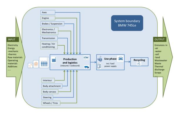
Fig. 1: Flowchart input / output data of the BMW 7series
