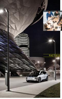
Electric vehicles in Munich, Oxford and Los Angeles can now also be charged at Lightand-Charge-streetlamps. The BMW Group's energyefficient LED streetlamps provide free charging up to 22 kW. Thermoplastic parts of the BMW i3 contain 25 per cent renewable natural and recycled materials. These are clearly visible and part of the driver experience – from naturally-tanned leather to a dashboard from certified eucalyptus wood to seat covers made from PET bottles.
