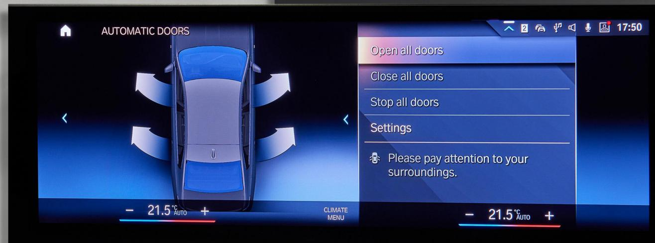
➤ Automatic doors with collision protection function.
