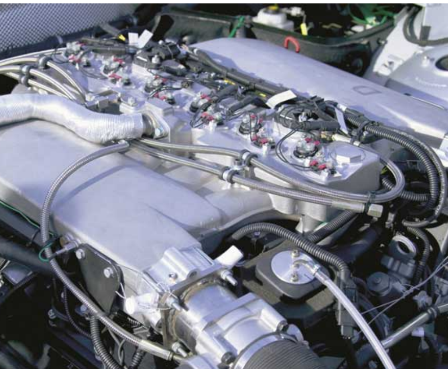
12 cylinders, six litres, 285 bhp: the hydrogen engine gives the H 2 R a top speed of more than 300 km/h.
